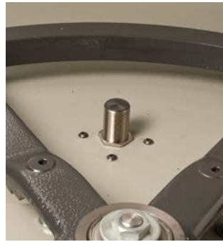
Safety Shutoff Sensor
